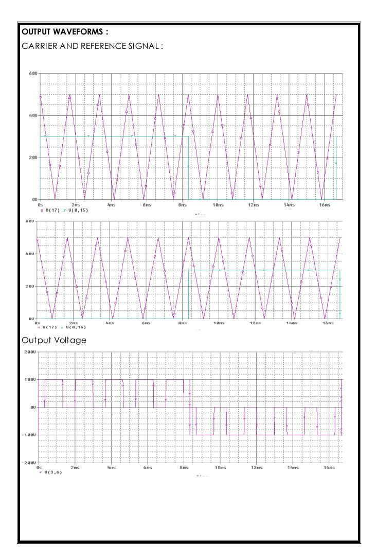
Rg4 14 13 100 \*subckt call for pwm control xpwm1 17 15 8 3 pwm xpwm21715100pwm xpwm3 17 16 12 6 pwm xpwm41716140pwm .subcktpwm1234 \*model ref carrier +control -control \*name input input voltage voltage R1151k R2251k Rin502meg Rf5 3 100k Ro 6375 Co 3 4 10pf E1 6 4 0 5.2e+5 .Endspwm .Tran 100us 16.67ms 0 10us .Probe .options abstol=1.00n reltol=0.01 vntol=0.1 ITL5=20000 .Four 60 v (3,6)
