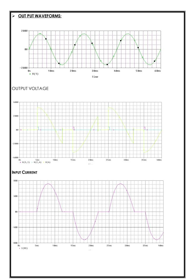
Theoretically the value of Extinction angle calculated by  $\beta$ = ( $\pi+\phi$ ); Where  $\phi$ =tan-1(wL/R)
