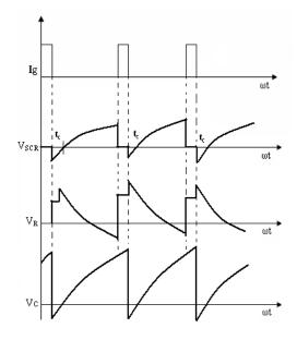
Voltages and currents in class B  $tc = SCR turn off time in \mu sec's$ .
